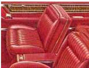
*This is the Fleetwood Eldorado Convertible with perforated leather seat cushions and seat-back inserts. A choice of bucket or bench type seats is offered at no extra charge. Shown here in red is one of the Eldorado's eight interior combinations.*
