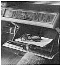
The newly designed and larger glove box (*left*) is now centrally located within easy reach of both driver and passenger. Twin ash receivers and lighter are concealed behind the wood-covered panel above this compartment.
