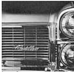
All metalwork both inside and outside the car is crafted with Cadillac perfection. The completely new grille (*left*), for instance, combines bright and satin finished chrome and is highlighted by the famous Cadillac script. Concealed behind the grille is the optional Guide-Matic headlamp control photo cell.
