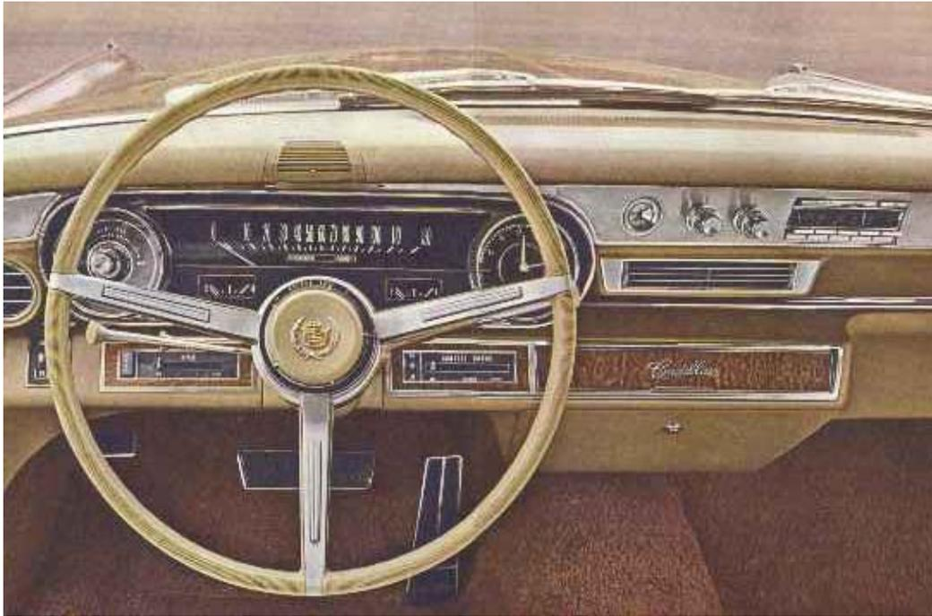
*COMFORT CONTROL: Combines heating and air conditioning in a single unit. A dial permits setting of interior temperature as easily as with a home thermostat. Once set, the temperature is automatically maintained regardless of changes in the weather or the season.*
