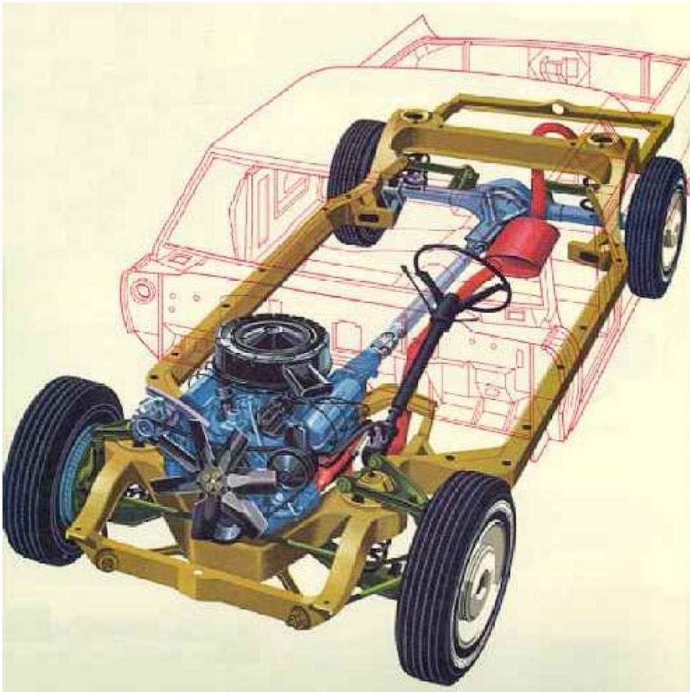
Cadillac continues to offer the industry's only true triple braking. There are independent front and rear braking systems, together with a foot-operated parking brake that can be used as an emergency brake while the car is in motion. All four brake drums are finned for better cooling and are self-adjusting.
