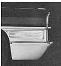
The cornering lights (*left*) are an integral part of the front bumper design. They are now larger and have been redesigned to provide improved illumination.
